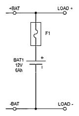
Circuit 3 is simply the battery. The battery is connected through the fuse into solar modules. So input from the solar modules will come through and into the battery (Assuming that circuit 2 is not active) and charge it. A fuse is present incase something goes wrong in other subsystems and excess power starts overfilling the battery. This subsystem is also connected to other systems allowing it to output into other systems and further the function.
