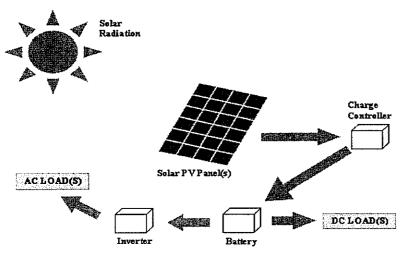
Diagram shows process of electricity through a solar charger and interaction between systems.
